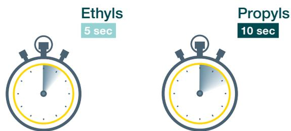
Ethyls evaporate about two-times faster than Propyls
