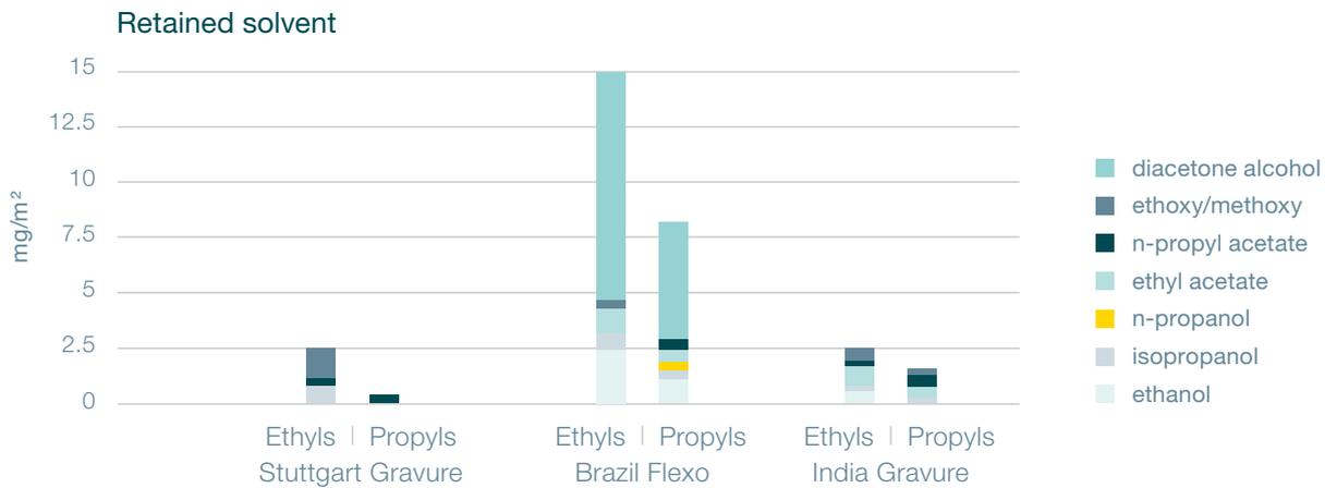
GC measurements in industrial scale trials clearly indicate the trend of less retained solvent while exchanging Ethyls by Propyls. This trend applies for both Flexo and Gravure.
