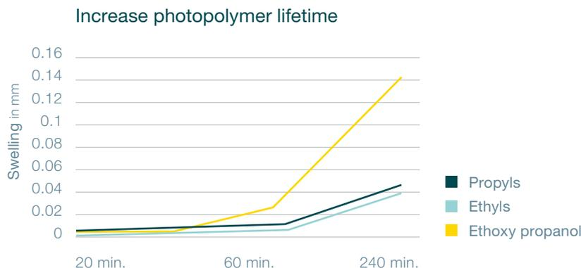
Ethyls blends require more Glycol Ether than Propyls blends. As Glycol Ethers are more aggressive against the photopolymer than linear alcohols, the reduction of such leads to a prolonged durability of the photopolymer.
