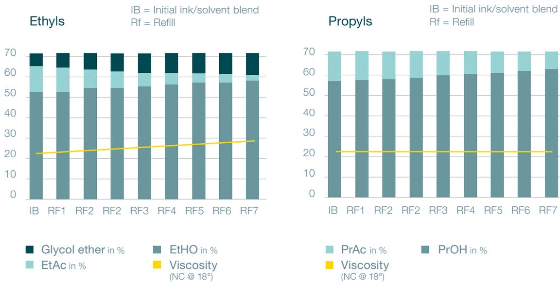
Refilling with alcohol-ester solvent blends in the course of printing shifts the composition towards lower ester content. Propyls facilitate a more consistent ink composition which has a direct positive impact on print quality. When using Ethyls thinners, the viscosity is negatively impacted due to its evaporation behavior. This calls for the addition of more thinner which in turn decreases color density.
