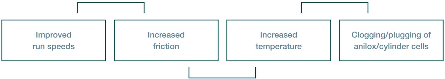
How increased printing speed leads to clogging/plugging
