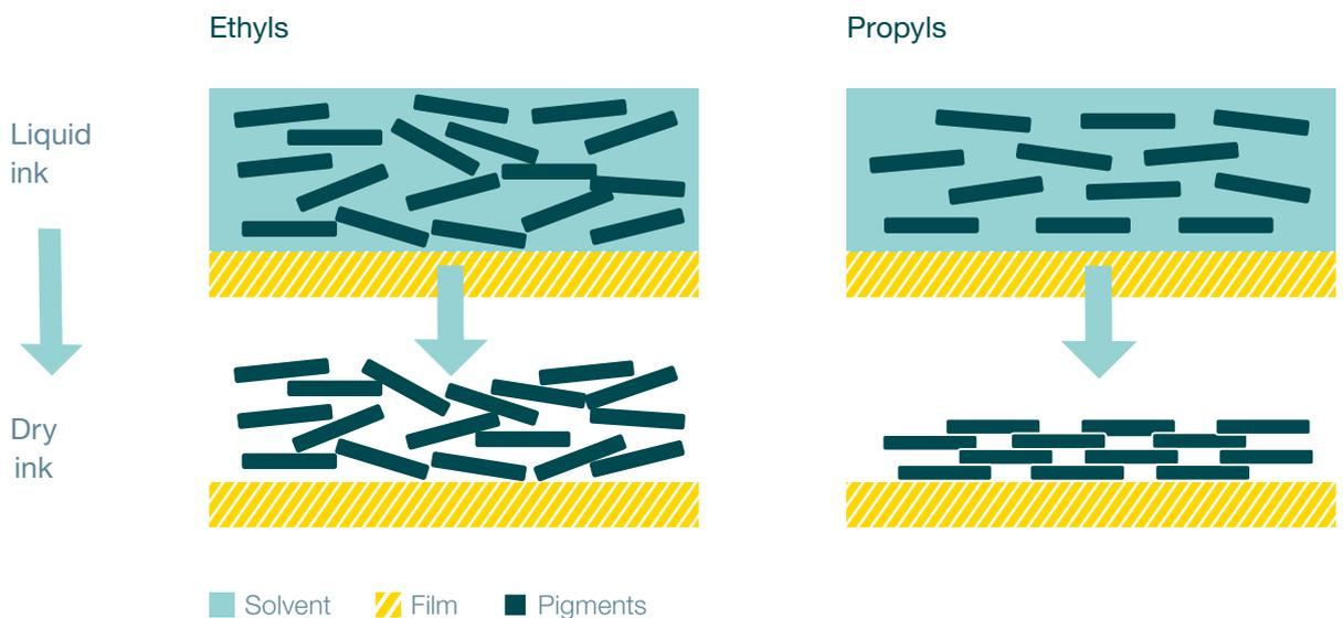
In the Ethyls solvent system (left side of the illustration) pigments do not distribute uniformly on the printing film while pigments build a homogenous layer due to their medium evaporation behavior (right side of the illustration).
