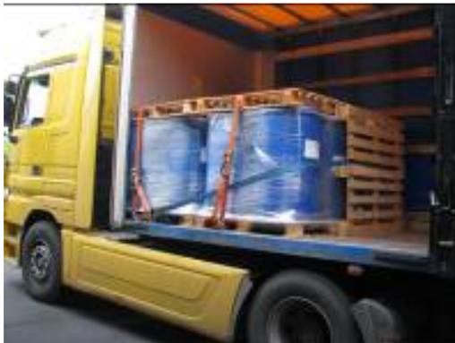
Direct lashing combined with lashing down
