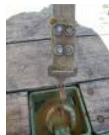
Defective lashing belts or defective/insufficient number of anchor points
